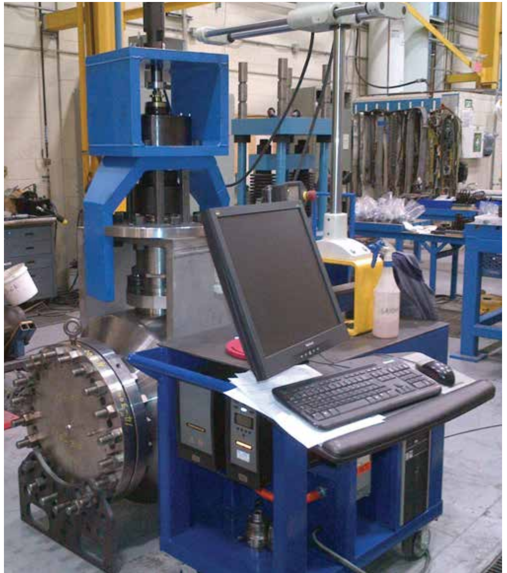
The above 16", Class 300, Type R Securaseal metal-seated ball valve is actuated with the direct mount 50,000 Nm +/- 7.5% unit, using Velan's mobile controller, and a bracket design. This allows for self-adjusting vertical motion, making it versatile to use on a large range of valve designs.
